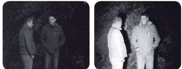
Observation without arousing suspicion at a distance of 80 m (left: without laser, right: with laser).
