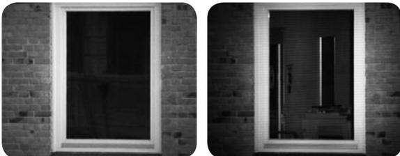
Left: Observation from a distance of 40 m without laser. Right: Observation from a distance of 40 m with laser: the inside of the room is visible.
