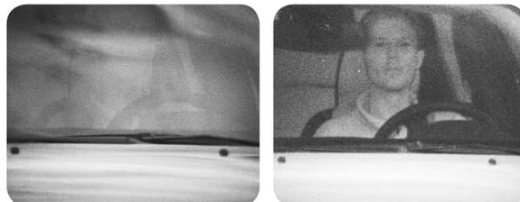
Interfering sunlight is reduced by special filters, whilst at the same time the scene is also illuminated with IR light.
